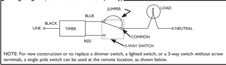
**Wiring diagram, 2 switch installation (3-way) using a single pole remote switch:**
