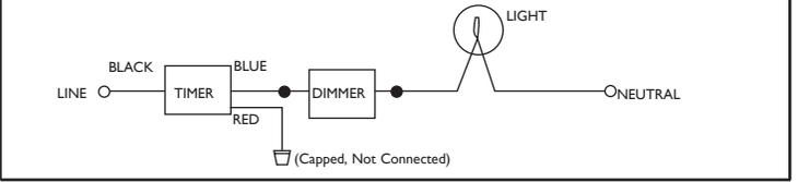
**Multi-switch installation using a dimmer :**
