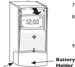
7. Pull at notch at top edge to remove the clear/cover switch so you can use the programming buttons.
