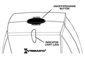
5. To manually turn OFF the **HA02 Appliance Module**, simply press and release the Program/ON/OFF button. The green indicator will turn OFF and the lamp or appliance plugged into the **HA02 Appliance Module** will also turn OFF.
