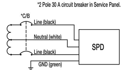
SPD TYPE 2 WIRING DIAGRAM
