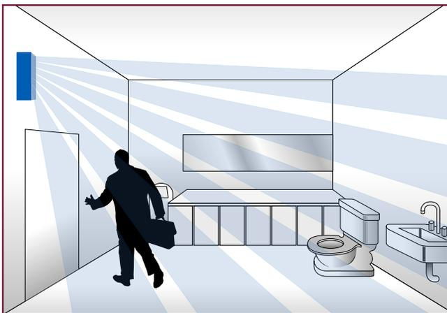
**Passive infrared (PIR) technology** detects the difference in heat energy a person in motion generates in contrast to the elements surrounding them in a confined space. To detect presence PIR needs line of sight to a person.
