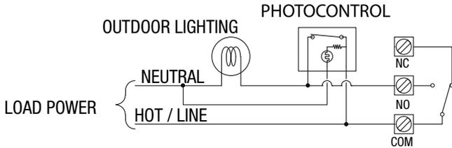
Typical installation for photocontrol in parallel with time switch contacts. Either the time switch OR the photocontrol must be ON to power the load. Ideal for improved safety. Loads will activate at the scheduled times, at night, or during low-light conditions such as a storm.
