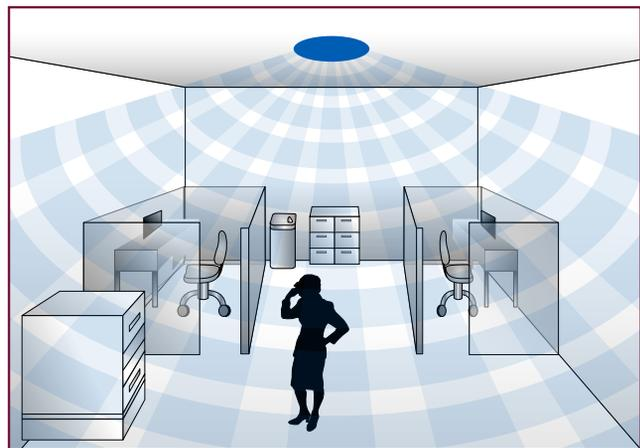
**Dual (PIR/Ultrasonic) technology** combines PIR with Ultrasonic technology. Ultrasonic utilizes wave analysis and Doppler sound waves to detect differences in energy from different phenomenon. The combination of the two technologies enhances responsiveness for maximum system reliability.
