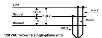
120 VAC Two-wire single-phase with separate ground. Found at connections for individual pieces of equipment such as pumps and single-phase motors. NOTE: Both Black wires connect to Line.
