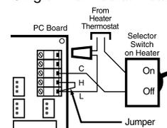
1. Connect two 18 gauge wires in SERIES with Heater's Selector Switches.
