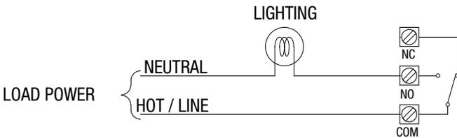
Typical lighting installation. Multiple loads may be wired concurrently, within the maximum output ratings for the circuit.
