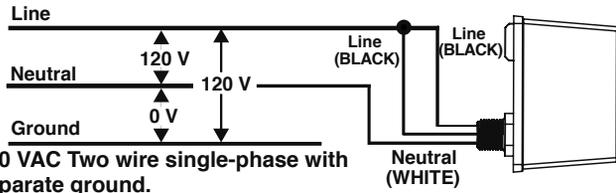
Found at connections for individual pieces of equipment such as pumps, single phase motors and HVAC applications.
