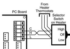
1. Connect three 18 gauge wires in PARALLEL with Heater's Selector Switches.
