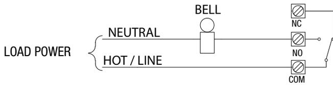
Typical bell, buzzer, or ringing installation. Multiple loads may be wired concurrently, within the maximum output ratings for the circuit.
