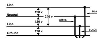
120/240 VAC Three-wire with separate ground. Found in Main Disconnect Switches, Main Distribution panels, Load Centers Sub panels and equipment locations.
